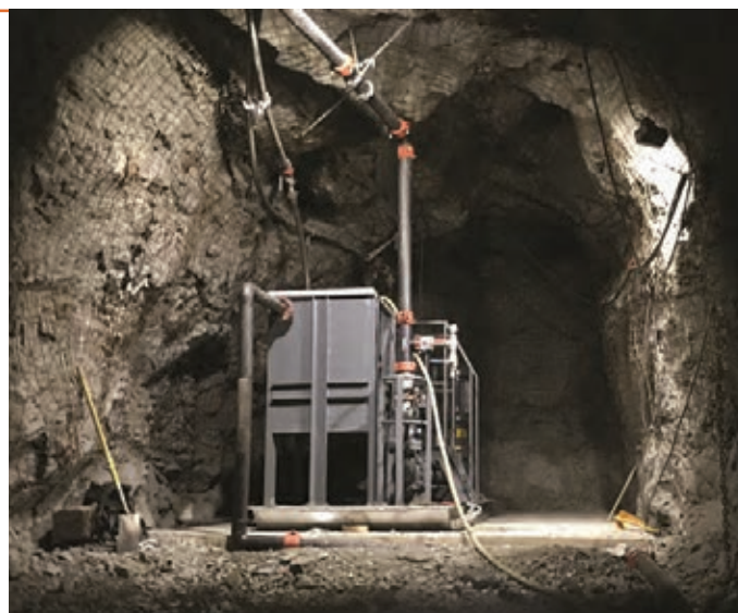
A Netzsch Mine Dewatering Skid in action
