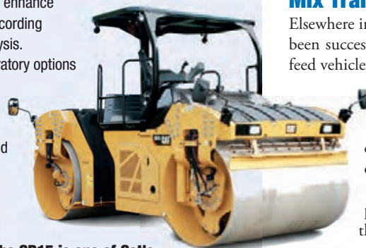
The CB15 is one of Cat's three new tandem vibratory rollers
