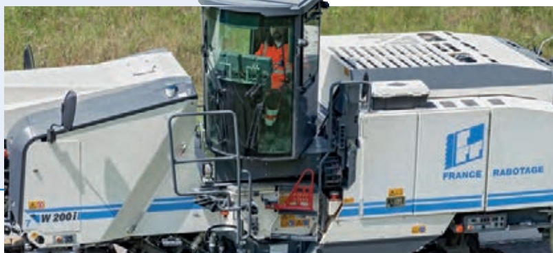
Wirtgen's new operator comfort system can be swivelled 110° in either direction
